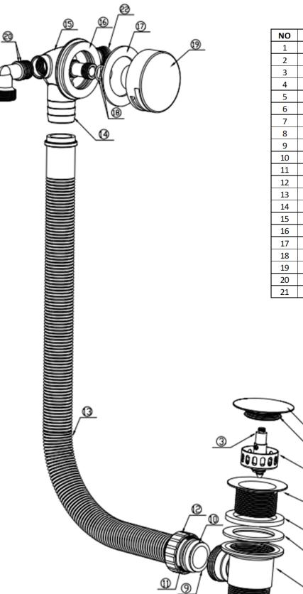
Description QTY Waste Cap 1 Washer 1 Click clack 1 Filter 1 Waste Cup 1 Washer 1 Washer 1 Waste 1 Thread 1 Seal washer 1 Washer 1 **Plastic nut** 1 Plastic pipe 1 Connector 1 3 way main pipe 1 Washer 1 washer 1 O-ring 2 Bath Filler Cap 1 **Filler connector** 1 flow elbow + O-ring 1
