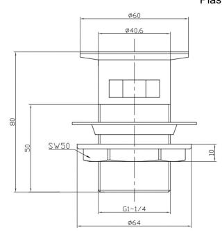
Brass body, cover cap and clic-clac spring (HPb57-3), equivalent to EN CuZn39Pb3 / CW614N Chrome plated to BS EN 248 Contemporary Min. 0.2 bar, Max. 5.0 bar Brass G1-1/4" **BSP** Male Thread (Outside Diameter 40.5+/ -0.25mm) 1 year against manufacturing faults (excluding serviceable parts) Size: 80 mm tall; Plastic lock nut
