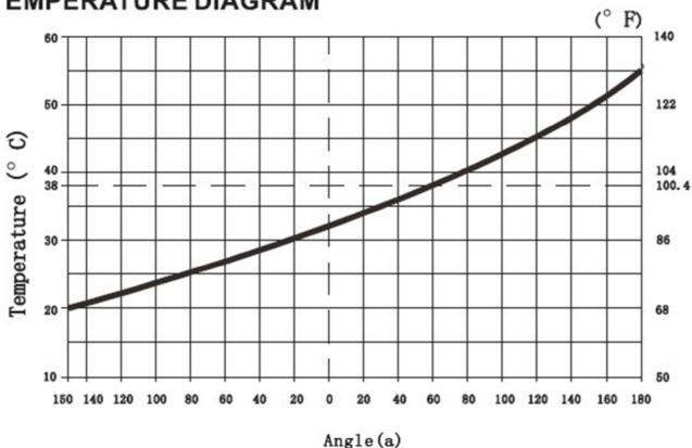
The optimum thermostatic temperature control range of mixer: 35°C~45°C(95°F~113°F).
