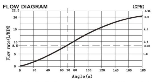
Flow rate @ 3bar(43.5psi) inlet pressure and 38°C (100.4°F) preset temperature curve is for reference only. The actual pressure drop may vary depending on inlet temperature and pressure.
