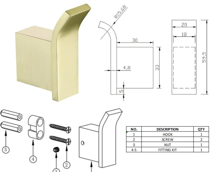
The information contained on this page was correct at the date of issue. Fitting dimensions are provided as a guide only. Some variation may occur due to manufacturing tolerances.
