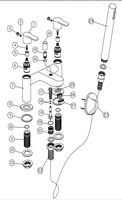
No. Description Qty Handle M5\*6 Screw Plastic Badge M4\*9 Screw PVC Core 3/4" Cartridge Body Base Plate 46#38#2.5 Rubber Vasher 24\*2.4 D-Ring 3/4" BSP Tails 3/4" Rubber Washer Plastic Back Nut Diverter Cap Connector 12\*2 0-Ring Spring **\*1.6** D-Ring Diverter Core 20\*2 0-Ring Hose Connector 150CM Flexible Hose Bracket Handhold Shower 23#15#3 Rub Washer Neoperl Aerator Nozzle
