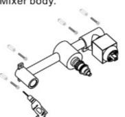
3.Refer to the diagram, locate and fit the plate by screwing outlet connector to the mixer body.
