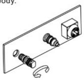
4. Adjust the Diverter and the flow cartridge to the right position and screw diverter body on.
