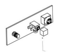
6.Screw the spout on after levelled . Make sure you protect the Chrome plated surface
