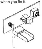
7. Screw the flow handle on and put the screw cap on afterwards.
